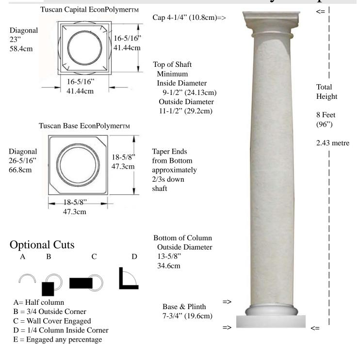
Weight Shaft 153 lb (69.4 Kg) Centered Load to 20,000lbs (9.07m tons)
