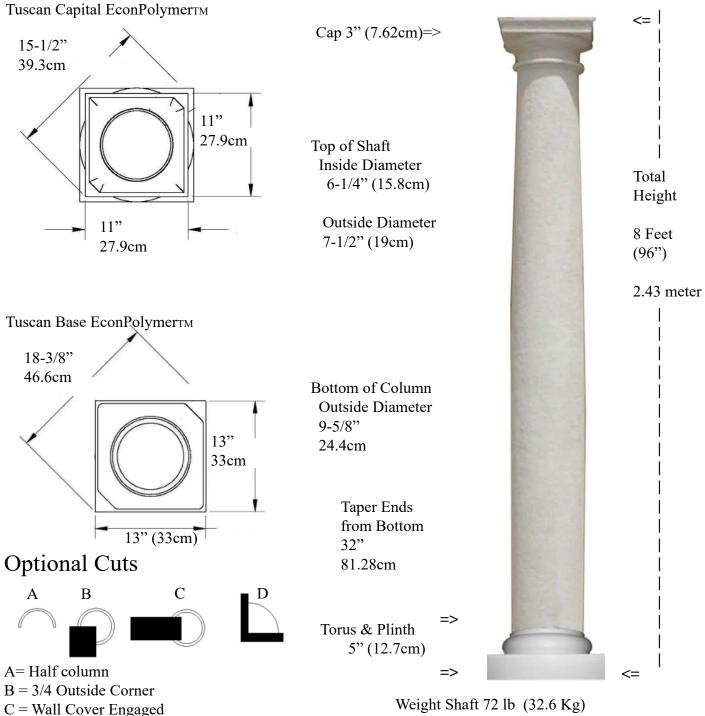
Weight Shaft 72 lb (32.6 Kg) Center Loads to 14,000lbs (6.35m tons)
