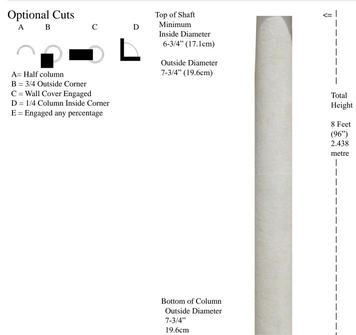
Shaft weight 61 lbs (27.6kg) Center Loads to 10,000lbs (4.53m tons)
